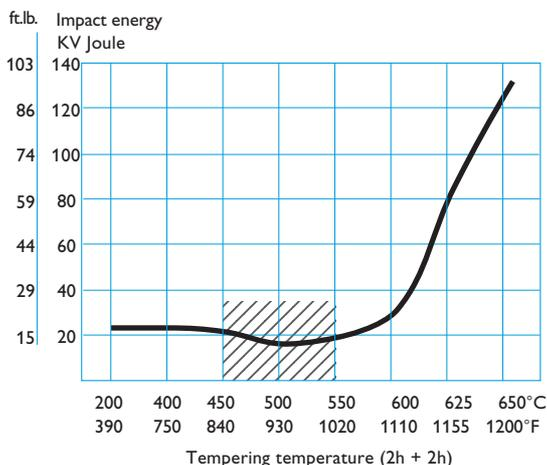
Tempering in the temperature range 450–550°C (840–1020°F) for the intended final hardness will result in a lower toughness.
