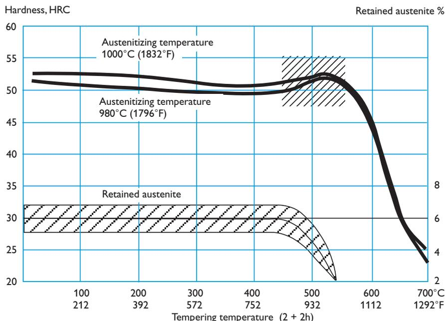
Above tempering curves are obtained after heat treatment of samples with a size of 15 x 15 x 40 mm, cooling in forced air. Lower hardness can be expected after heat treatment of tools and dies due to factors like actual tool size and heat treatment parameters.
