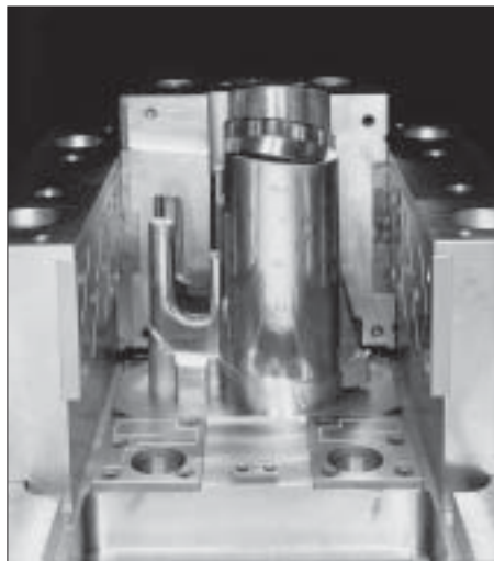
A highly polished mould in Uddeholm Stavax ESR which produces the body for an electric kettle.
