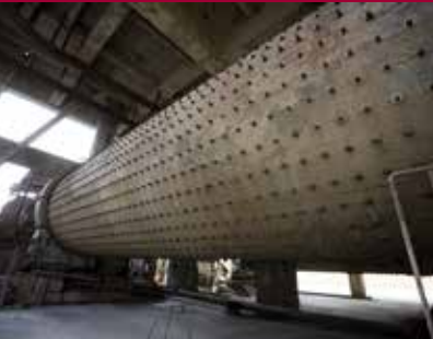
Ball mills Hardox 500, 550 or 600 are the recommended materials for wear protection at the inlet and outlet in ball mills.
