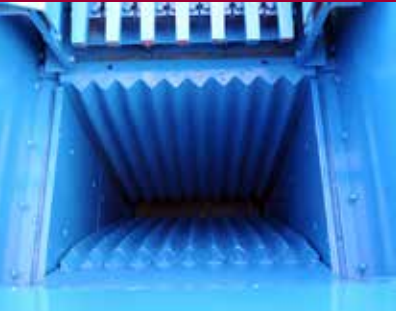
Jaw crusher For the cheek plates in a jaw crusher Hardox 500, 550 and 600 are all suitable to battle the wear and impact loads generated by crushing limestone.
