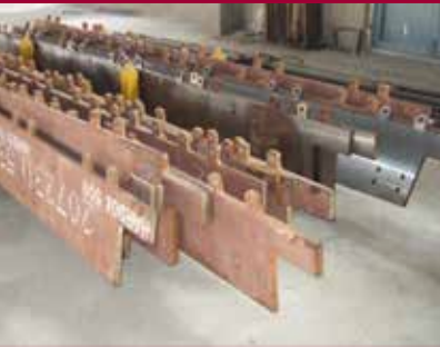
Guide plates Hardox 500 is the common choice for guide plates in the clinker cooling bed.
